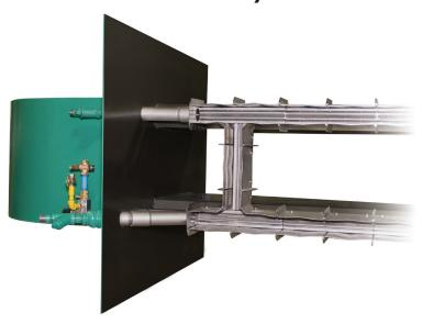
combinations of modules and rows, a wide range of inputs and footprints can be achieved. Because of the modular burner design, standard burners can be assembled in lengths from 0.91 m to 2.7 m (3 to 9 feet) with 1 foot modular sections ranging from 90 - 2700 kBtu/h each. In addition, multiple rows of these modules can be used, which greatly increases burner capacity as well as ability to adapt to nearly any application.
