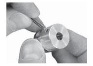
1. Insert the 3mm spring pin partially into the coupling. Insertion may be easier by first squeezing the tip slightly with pliers.
