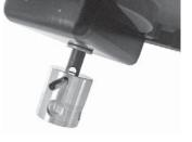
2. Install the coupling onto the actuator shaft and align the drive hole in the coupling with the through hole in the shaft. A view from the hole on the backside will assist alignment.
