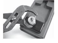
3. Use slip-lock pliers to press the spring pin through the coupling and shaft. Make sure the actuator body is supported and be careful not to apply excessive stress on the shaft.
