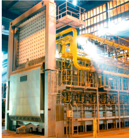
Bogie hearth forging furnace
