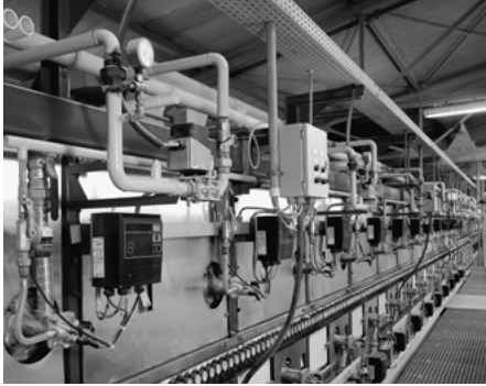
Roller hearth kiln in the ceramics industry
