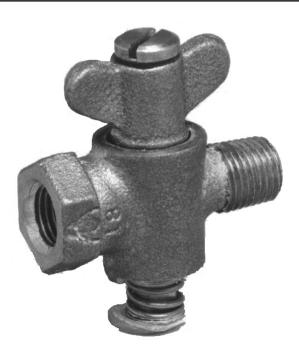
Pressure: 1/2 psig Cv: 0.3 Full open rating for natural gas at 0.6 sg Natural Gas Flow at 1" w.c. drop: 17 cfh End-to-End Length: 1-3/4" Material: Brass Thread Size: 1/4" NPT female x 1/4" NPT male Part Number: 12659
